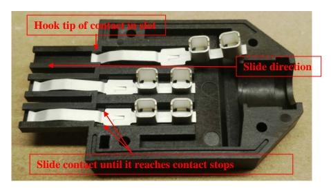
• It is important to never use die-electric grease on the contacts. Grease can hold in dirt and debris not allowing the connector contacts to make a good electrical contact. We recommend using WD-40. Simply spray the contact down and then blow out any excess with compressed air. This will wash out any dirt and apply a protective coating to each contact.
