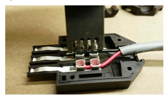
Once the wires have been inserted into the clips it is very important to solder the bared ends of each wire. This will insure a good connection to each contact clip. If needed, electrical tape or thin single wall shrink tube can be added to the ends of exterior jacket to ensure a tight clapping fit with the strain relief insert.
