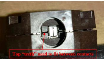
• Should a contact fall out of the bottom simply slide the contact back into its holder. Start by hooking end of the contact back into the t-slot and slide the contact until it reaches the stops in the plastic bottom.
